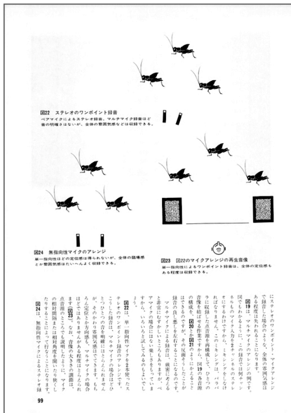
Fig.4 Illustrations of a microphone arrangement based on the classification between point, group, moving sound source, by Minoru Gennaka. Tape Sound , no.11, 1973, p.99.
